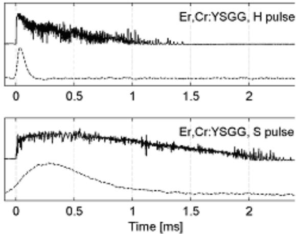
Fig. 19: Measured temporal evolutions of the output laser radiation (full line), and flashlamp pump optical emission (dotted line) for an Er,Cr:YSGG laser system (Waterlase MD, H and S pulse mode). Data is from ref. 18.
