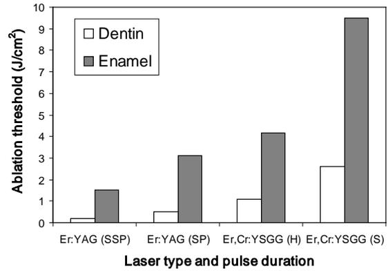
Fig. 14: Dependence of the ablation threshold in enamel and dentin on the pulse duration and laser type. The ablation threshold for the shortest SSP (50  $\mu$ s) Er:YAG (Fotona dental laser) laser pulse is by a factor of 3 lower compared to that of the H (500-700  $\mu$ s) Er,Cr:YSGG laser pulse, and by a factor of 6 lower compared to the S (1600-2000  $\mu$ s) Er,Cr:YSGG laser pulse (Biolase Waterlase). Figure is based on data from ref. 8.
