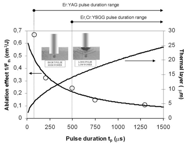
Fig. 12: a) Dependence of thermal effects on laser pulse duration as represented by the thickness of the thermally affected layer in enamel. b) Dependence of ablation effect, represented by the inverse of the ablation threshold fluence in enamel on laser pulse duration. Circles represent experimental data from Fig. 13, the full line represents  $1/x$  fit. Due to the long population inversion time of Er,Cr:YSGG, this laser cannot be operated below approximately 500 µs.
