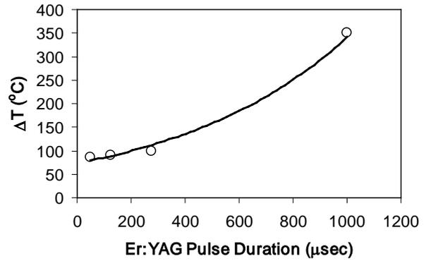
Fig. 25: Enamel surface temperatures 2.5 ms following a laser pulse for different VSP Er:YAG pulse durations (Fotona dental laser, pulse durations SSP, MSP, SP and VLP). Figure is based on data from ref. 42.
