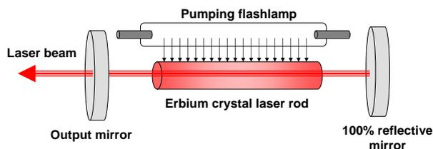
Fig. 2: A typical simplified Erbium laser configuration.
