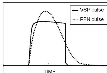
Fig. 18: Temporal shape of the VSP (full line) and PFN (dotted line) current pump pulse. Data is from ref. 43.
