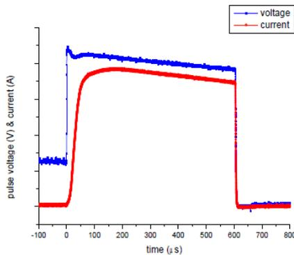
Fig. 4: Temporal development of the flashlamp voltage and current during a VSP flashlamp pulse of duration 600  $\mu$ sec. Note that the current pulse duration is not defined by the rise and fall times but with the on and off time of the switching transistor. The VSP pulse is almost “square shaped”, with the full width half max range of the pulse slightly closer to the end of the pulse. The Figure is based on data from references 43.
