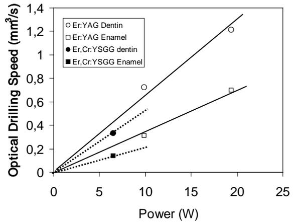
Fig. 23: Plot of measured results of drilling speeds in dentine and enamel for VSP Er:YAG (Fotona dental laser, MSP mode) and Er,Cr:YSGG (Biolase Waterlase, H mode). Figure is based on data from ref. 8.
