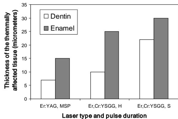
Fig. 15: Measured depths of thermally affected layers in dentin and enamel for Er:YAG (Fotona dental laser, MSP) and Er,Cr:YSGG (Bioalase Waterlase, H and S). Figure is based on data from ref. 18.
