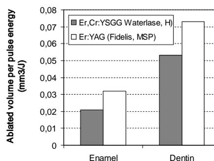
Fig. 10: Plot of measured results of ablated volume per pulse energy of dentine and enamel for both laser sources at 260 mJ pulse energy. The figure is based on data from ref. 8.
