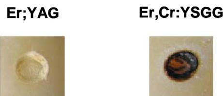
Fig. 9: Pictures of cavities in dentin, made with Er:YAG and Er,Cr:YSGG lasers following three consecutive laser pulses of the same laser pulse fluence of  $80 \text{ J/cm}^2$  [19]. In order to eliminate any influence of the difference in pulse duration, the Er:YAG pulse duration (Fotona dental laser, VSP mode) was adjusted to match that of the Er,Cr:YSGG (Waterlase PFN S mode). In this experiment, no water spray was used.
