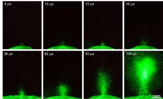
Fig. 20: Cloud images at different delays from the onset of an Erbium laser pulse. Cloud formation time is approx. 50-150  $\mu$ sec. Figure is reprinted with permission from ref. 40.
