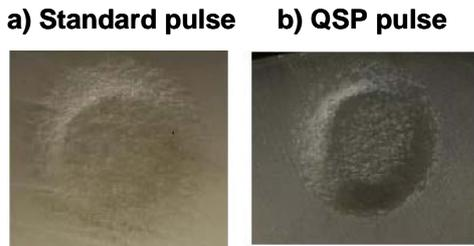
Fig. 22: Comparison of the quality of laser-ablated cavities in dentin with a high energy Erbium pulse and with a QSP Er:YAG pulse of the same pulse energy. Note the difference in the ablated depth and the sharpness of the cavity edges. Figure reprinted with permission from ref. 40.
