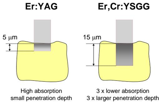
Fig. 6: Because of the higher absorption, the Er:YAG laser has a smaller penetration depth, and therefore requires less energy and less time to ablate the tissue. The shown penetration depths are for dentine.
